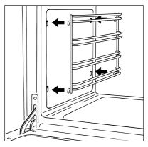
Fig.36 Removing the side racks
